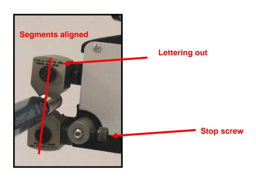
4. Depress the upper arm lever to raise the upper segment. Tighten the axis screw in the upper segment and then back off just enough so the segments can move freely.
