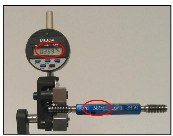
7. Press the lever downward. Remove the GO set plug and insert the NOGO set plug between the segments. Rotate the set plug slightly to assure it is seated completely between the segments and observe the indicator reading.
